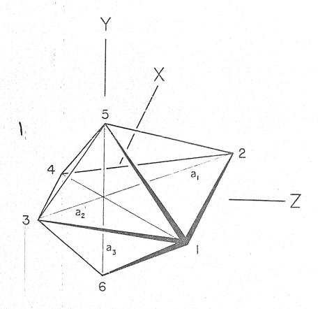
Figure 1. Idealized  $C_{2v}$  coordination site in which Z, the two-fold rotation axis, is a dihedral axis. Points 1 through 6 have  $(r,\theta,\phi)$  coordinates of  $(a_1,\theta_1,\pi)$ ,  $(a_1,\theta_1,0)$ ,  $(a_2,\theta_2,\pi)$ ,  $(a_2,\theta_2,0)$ ,  $(a_3,\theta_3,\pi/2)$  and  $(a_3,\theta_3,3\pi/2)$ , respectively.
